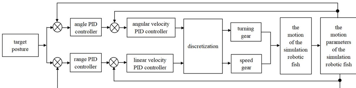
**Figure 2.** The simulation robotic fish posture control schematic diagram based on cascade PID.
