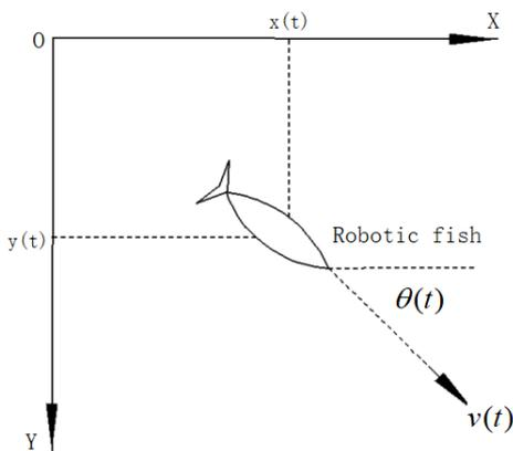
**Figure 1.** The motion simulation diagram of the robotic fish.
